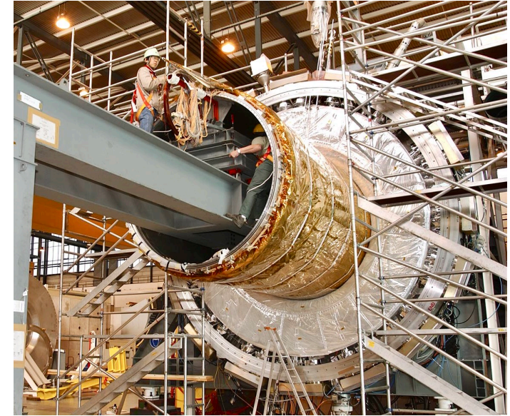
Insertion of ATLAS and CMS solenoids
