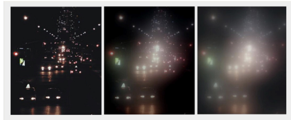
Multiple scattering (diffusion) of light passing through a wetter and wetter windscreen (left to right)
