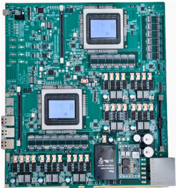
New ATLAS L0 Global Trigger: offline-quality reconstruction using input from calorimeters and muon systems built upon digital improvements realised during Phase-I upgrade
