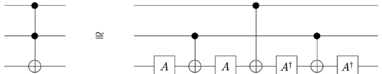
where  $A = R_y(\frac{\pi}{4})$ . In the above, the “ $\cong$ ” indicates that the networks are not identical, but differ at most in the phases of their amplitudes, which are all  $\pm 1$  (the phase of the  $|101\rangle$  state is reversed in this case).
