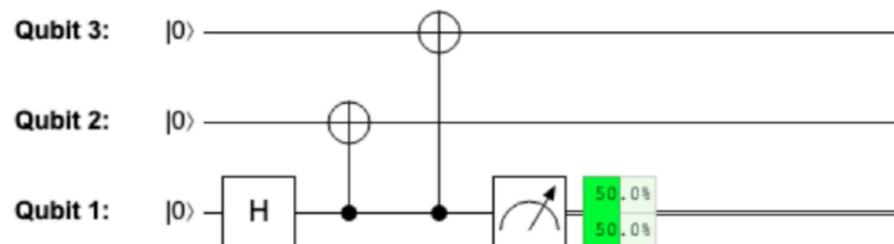
$$\hat{\text{CNOT}}_{1 \rightarrow 3} \hat{\text{CNOT}}_{1 \rightarrow 2} \hat{H}_1 |000\rangle = \frac{1}{\sqrt{2}} \left( \hat{\text{CNOT}}_{1 \rightarrow 3} \hat{\text{CNOT}}_{1 \rightarrow 2} |000\rangle + \hat{\text{CNOT}}_{1 \rightarrow 3} \hat{\text{CNOT}}_{1 \rightarrow 2} |100\rangle \right) = \frac{1}{\sqrt{2}} (|000\rangle + |111\rangle)$$
