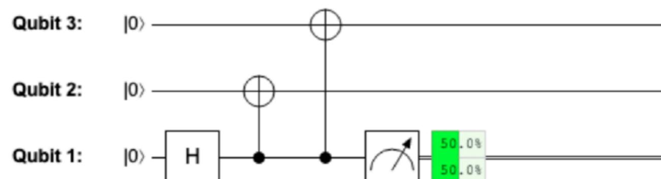
$$\hat{\text{CNOT}}_{1 \rightarrow 3} \hat{\text{CNOT}}_{1 \rightarrow 2} \hat{H}_1 |000\rangle = \frac{1}{\sqrt{2}} \left( \hat{\text{CNOT}}_{1 \rightarrow 3} \hat{\text{CNOT}}_{1 \rightarrow 2} |000\rangle + \hat{\text{CNOT}}_{1 \rightarrow 3} \hat{\text{CNOT}}_{1 \rightarrow 2} |100\rangle \right)$$
