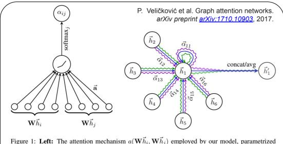
Figure 1: Left: The attention mechanism  $a(\mathbf{W}h_i, \mathbf{W}h_j)$  employed by our model, parametrized by a weight vector  $\vec{\mathbf{a}} \in \mathbb{R}^{2F'}$ , applying a LeakyReLU activation. **Right:** An illustration of multihead attention (with K = 3 heads) by node 1 on its neighborhood. Different arrow styles and colors denote independent attention computations. The aggregated features from each head are concatenated or averaged to obtain  $\vec{h}'_1$ .
