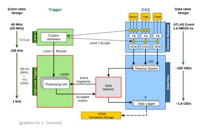
Hardware trigger (LVL1) • Decision in  $\sim 2.5 \,\mu s$ • Retains  $\sim 100 \, \text{kHz}$ High level trigger (HLT) • Offline-like algorithms • Decision in  $\sim 500 \,\mathrm{ms}$ • Max. 8 GB/s output  $\sim 3 \, \text{kHz}$  of full events  $\sim 5 \, \text{kHz}$  of 'partial' events
