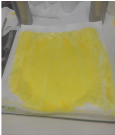
Coating the NOL film on Tyvek
